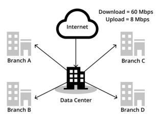
In summary, the bonder create an IP pipe between the cloud and the branch office, which has a capacity of 60Mbps from the cloud to the branch office, and a capacity of 8Mbps from the branch office to the cloud.
